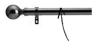
For both headings simply measure from the top of the pole to your chosen end point:
